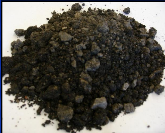
Reclaimed Asphalt Pavement
