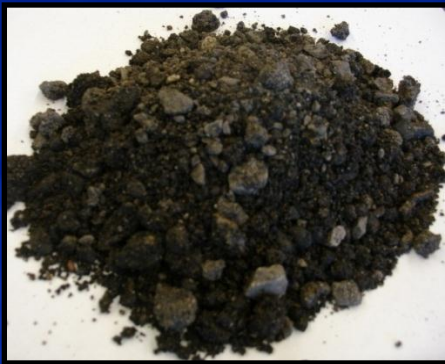
Reclaimed Asphalt Pavement
