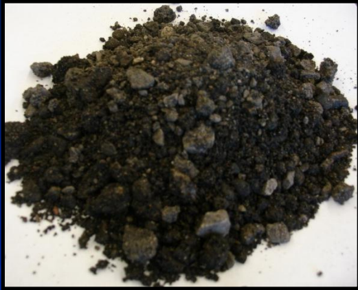
Reclaimed Asphalt Pavement
